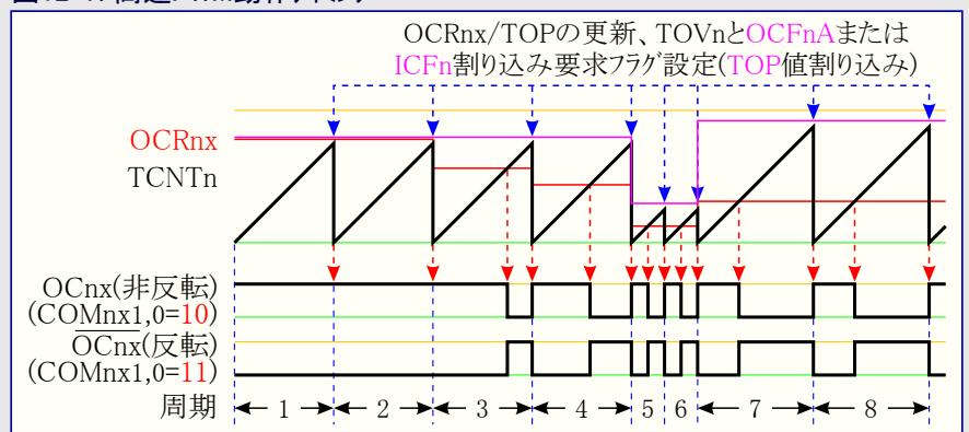
$$f_{\text{OCnx PWM}} = \frac{f_{\text{clk\_I/O}}}{N \times (1 + \text{TOP})}$$
